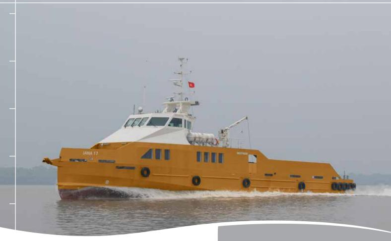
Concentrate of 25 years experience in fast crew boats, the FPSV 41P is designed with seating for 80 personnel and a cargo deck of 100 m<sup>2</sup>. She is the perfect vessel for operations such as rig crew transfer, quick transportation of supplies and in field support.
